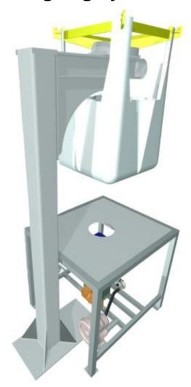
Resting column for big bag & yoke using existing lifting arrangements on site
