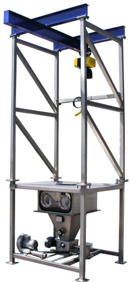
Elephant BBS big bag system is delivered in several configurations and consists of components that are also supplied separately:
